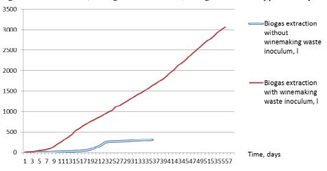
Fig. 2. Biogas output with and without winemaking waste inoculum
