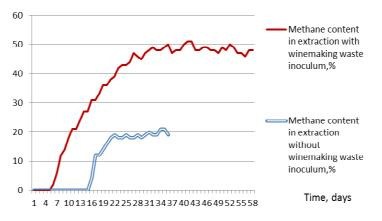
Fig. 3. Methane content in biogas with and without winemaking waste inoculum
