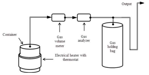
Fig. 1. Biogas digestion installation
